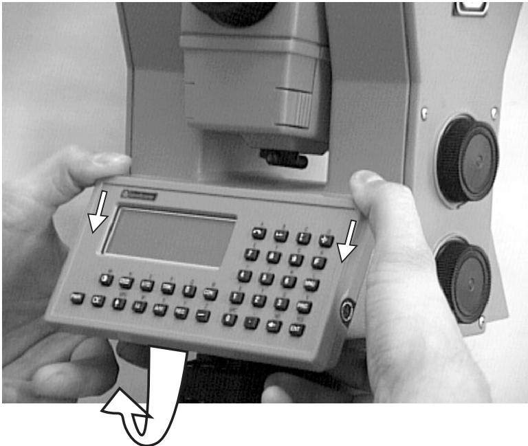
Fig. 1.4 How to attach/detach the control unit
