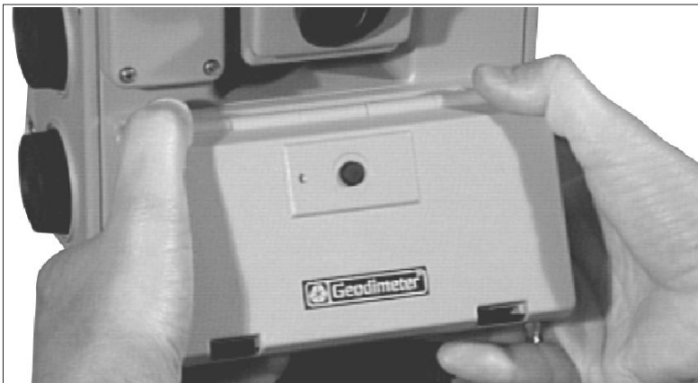
Fig 11.2 How to attach the card memory on an instrument.
