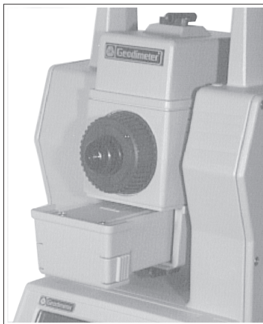
Fig. 3.1 Fitting the internal battery
