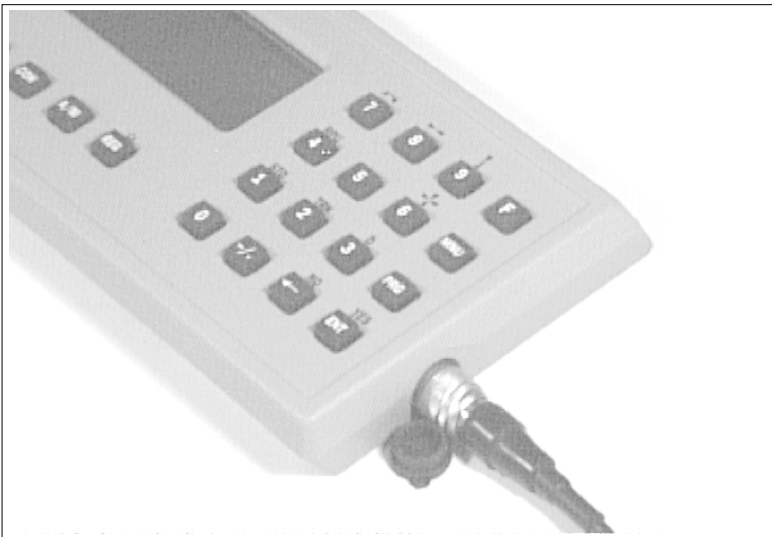
Fig 2.2 Connecting the external battery to the control unit.
